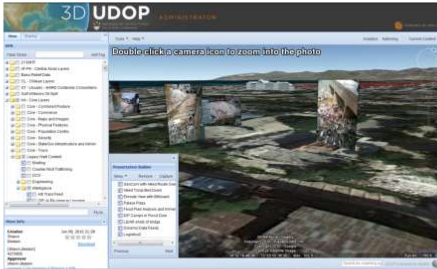
Figure 15 Disaster Relief and GEOCAM allow Smartphone users to upload images to the UDOP in real time providing immediate ground-truth analysis oriented in the direction the collector was facing. This on-scene information can be viewed in a user-defined presentation along with the rest of the UDOP's static and dynamic content.
